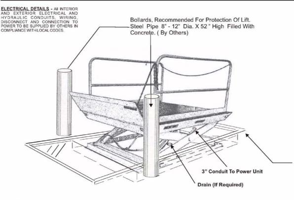
Note: For Floor Mounted Installation (Not Shown), Concrete Pad To Be Minimum 6" Wider and 6" Longer Than Dock Lift, And Concrete Pad To Be 8" - 10" Thick With Embedded Rebar, By Others And In Compliance With Local Codes,
